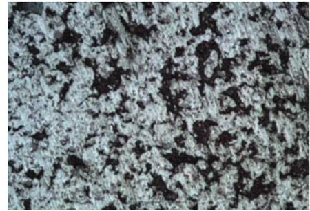
*Ceramic tip after alumina wear test*
