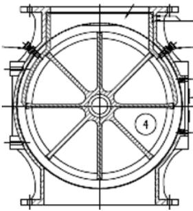
*Cut-away of an Anval Rotary Floating Shoe (RFS) valve*
