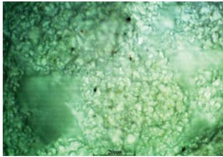
*Ceramic tip prior to alumina wear test*
